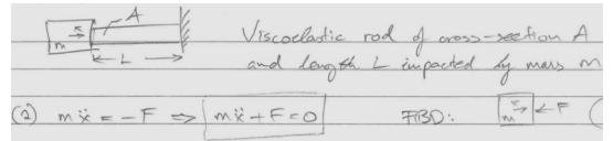
b) Assume that the free end of the rod is subjected to cyclic loading with  $x = x_0 e^{i\omega t}$  (i.e. replace the displacement in the equation of section (a) using the new expression given for the displacement). Rewrite the equation of motion in terms of stress and strain and solve for their ratio ( $\sigma/\varepsilon$ ).
