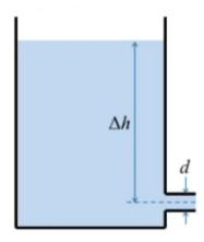
Derive an equation for the volumetric flow-rate (Q) through this pipe as a function of the fluid height. Assume that the flow is steady and friction does not play a role.
