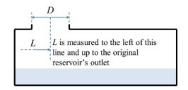
One can assume that the horizontal component is constant, which is the flow rate and the velocity. Since the position x is a function of the velocity at time t, one can say that  $x = v \cdot t$ Rewriting this gives us  $t = \frac{x}{v}$ . One can also say that x = L, giving us  $t = \frac{L}{v}$ . combining this into one equation gives us  $y = \frac{gt^2}{2} \rightarrow \frac{g(\frac{L}{v})^2}{2} \rightarrow \frac{g}{2}\frac{L^2}{v^2}$
